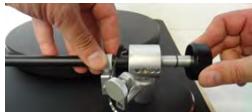
Pic. 2: Installing the counter weight
