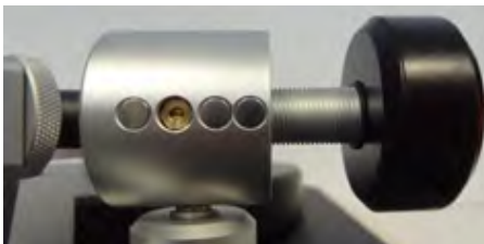
Pic. 3: Final position of the counter weight
