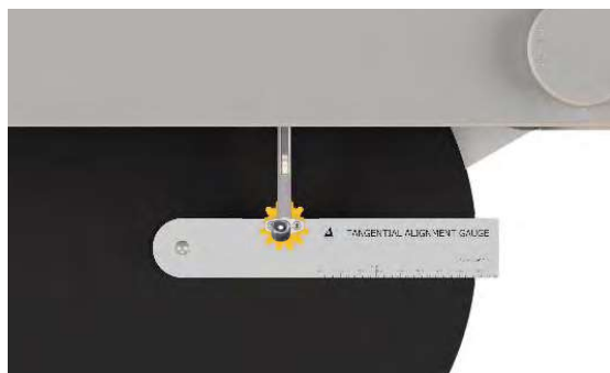
Pic. 14: Adjustment of the VTA
