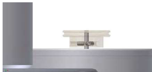
Pic. 21: Setting the motor pulley
