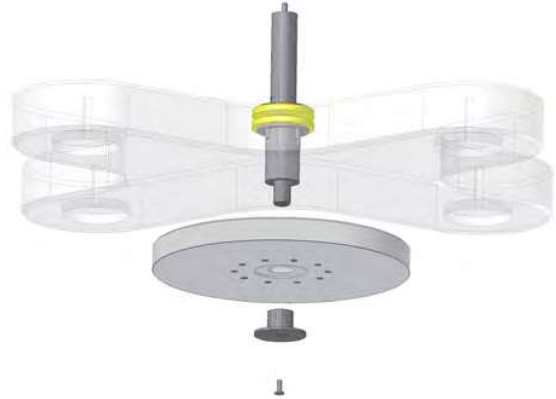
Pic. 15: To insert the bearing spindle into the bearing sleeve
