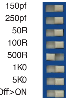
Pic. 2.3: Adjustment 500 Ohm, Subsonic "ON"
