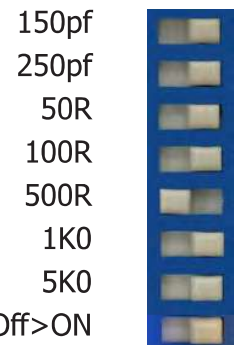
Pic. 3.3: Adjustment 500 Ohm, Subsonic "ON"
