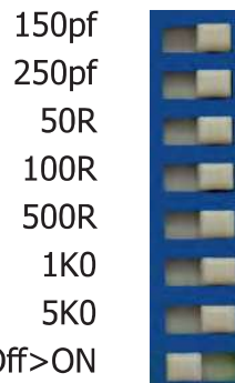
Pic. 3.2: Initial setting (150 pf - 5K0 "OFF", Subsonic "OFF")
