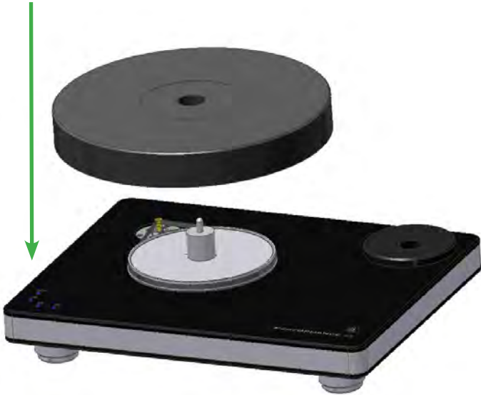
Pic. 8: Setting the platter onto the bearing
