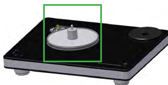
Pic. 7.1: Placing the belt
