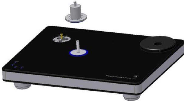
Pic. 6: Fitting the bearing upper part
