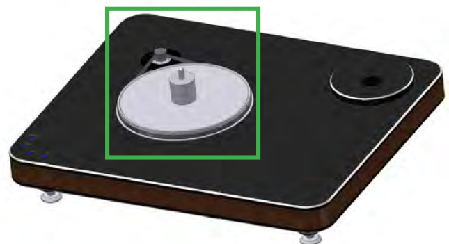
Pic. 7.1: Placing the belt
