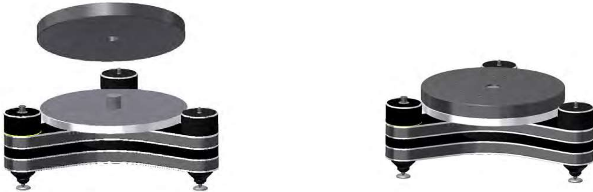
Pic. 9: Placing the drive unit platter onto the bearing
