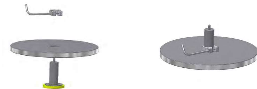
Pic. 7: Connection sub-platter and bearing upper part
