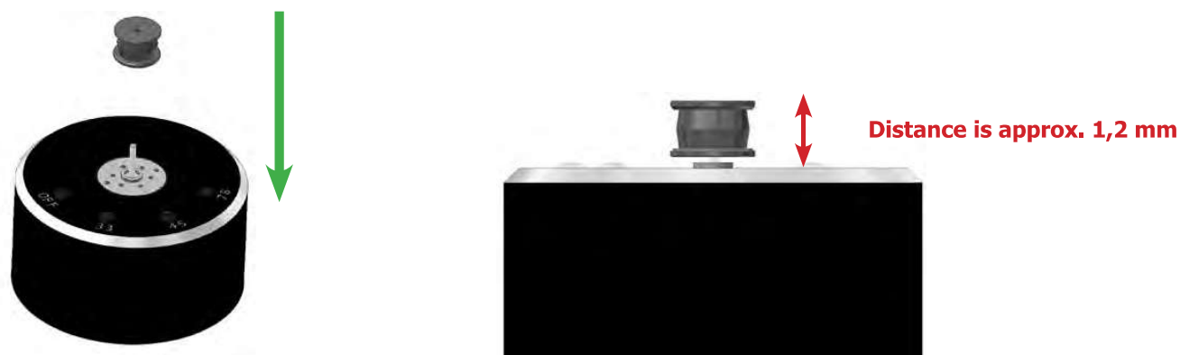
Pic. 10: Setup of the Master Innovation pulley
