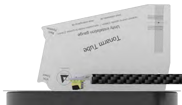
Pic 17: Parallelism of the tonearm tube
