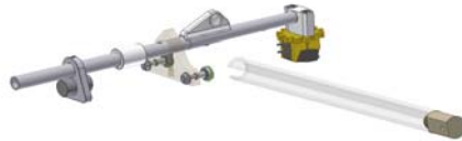
Picture 12: Placing the glstube into the precision tube holder
