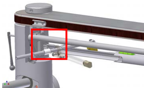
Picture 14: Fixing the tonearm with a tape
