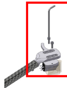
Pic. 5: Mounting the cartridge
