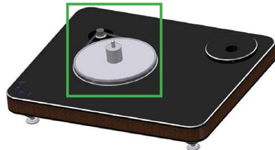
**Pic. 7.1:** Placing the belt
