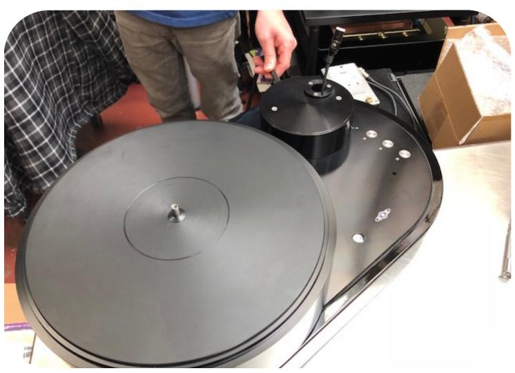
Connect tonearm cable to the AMG tone arm and gently place tonearm into the collar while pulling the tonearm cable the opposite direction back through the slot. If you are using the 12JT "Turbo" tonearm, loosen the VTA lock using the thumb screw located at the back of the tonearm. If this isn't loosened first, the tonearm will not drop fully into the mounting collar.
