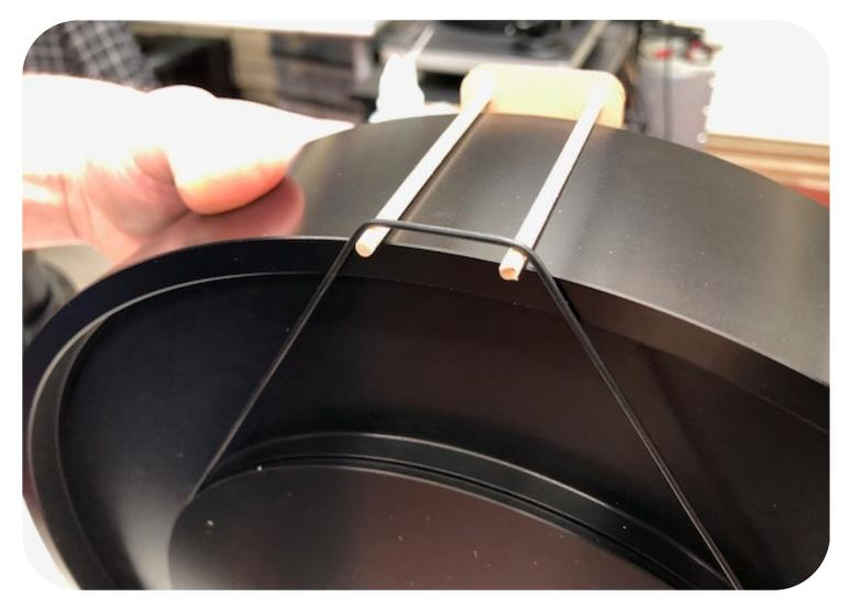
Set up shims laterally on the Viella table at both the 12 o'clock and 6 o'clock positions. Gently pick up the platter bracing the BMT with your right thumb - the two posts should be at the 2 o'clock position. You'll see that the motor pulley is positioned at that same 2 o'clock on the Viella plinth. Since the bearing is completely enclosed, no lubricant is needed on the bearing.
