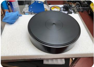
Get all the tools you'll need to properly set up the platter: two shims, belt mounting tool (BMT) and belt. Place the BMT over the platter spindle through the hole on the on the BMT with the posts on BMT facing downwards over the edge of the platter.
